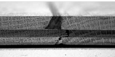
Milled groove for a wooden list.
